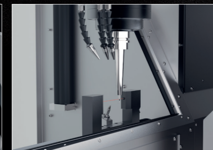
The laser measurement is outside the working range and prevents incorrect measurements due to contamination.
